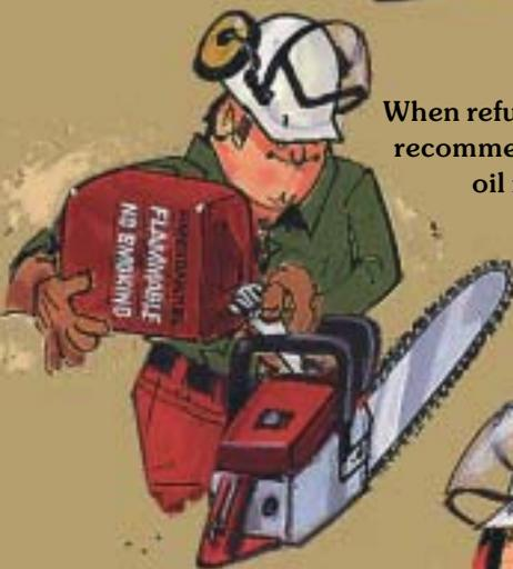
After refuelling, tighten the tank cap to prevent fuel spilling onto clothing
