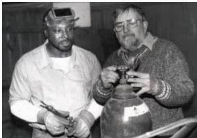
Building maintenance technology instructor Keith Goodin, right, and new graduate Harold Lewis inspect the pressure of an oxygen/acetylene tank before beginning a metal cutting project at the Jess Dunn Skills Center, Taft.
