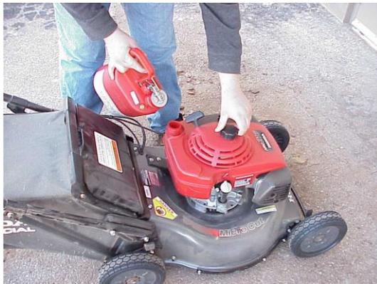
Fuel up outdoors and away from the grass. Be sure to wipe up all spills. Never refuel a running or hot engine. If you have been mowing and you run out of gas, let the mower cool down for several minutes before you begin refueling.
