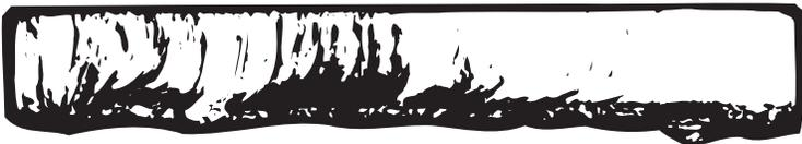
6. Pronounced break in the drag line with irregular cut edge and excess slag
