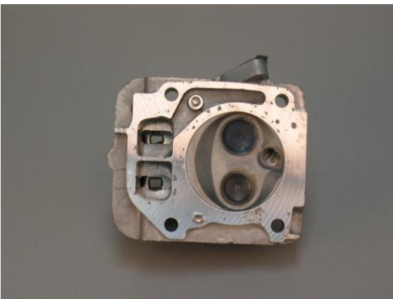
Combustion Chamber: the volume of the cylinder above the piston with the piston at top dead center.
