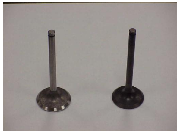
Intake Valve: a valve that permits the air- fuel mixture to enter the combustion chamber and seals its exit.
