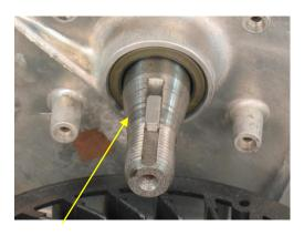
**Flywheel Key:** a device that holds the flywheel in place.
