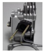
**Cylinder Head:** a detachable portion of an engine fastened securely to the cylinder block that contains all or part of the combustion chamber.
