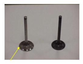
**Intake Valve:** a valve that permits the air-fuel mixture to enter the combustion chamber and seals its exit.
