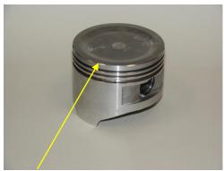
**Piston Head:** the part of the piston above the rings.
